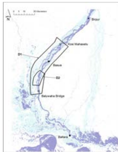
Figure 1. Model domains and gauges for the initial hydrodynamic and sediment models of the middle Kosi river.
