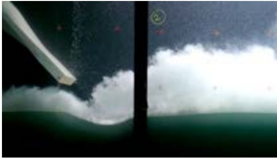
Figure 2. Scour result after approximately 23 seconds from the start of the experiment (snapshot E, Figure 1).
