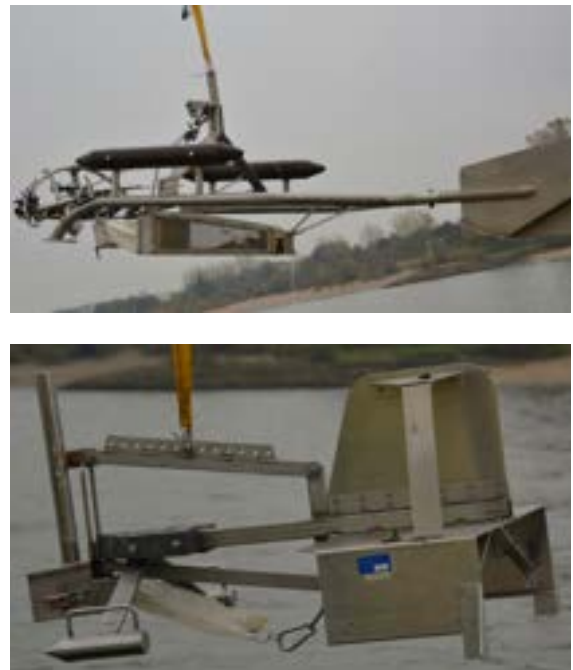
Figure 1. Improved Arnhem Sampler, as used by the German authorities (top) and Delft Nile Sampler, as used by the Dutch authorities (bottom). Note the difference in mesh size and the sample container.
