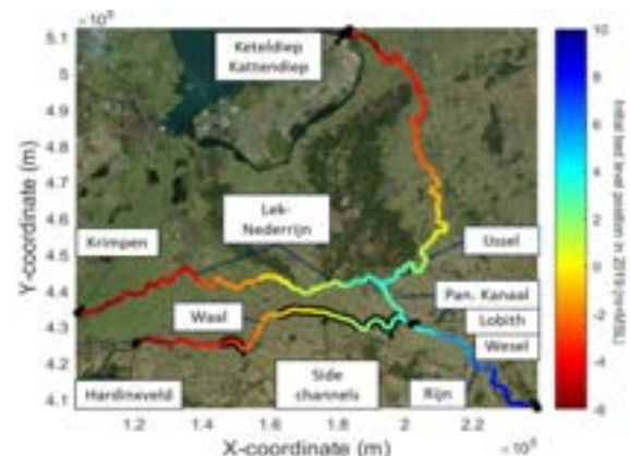
Figure 1. Model domain of the 1D-model including initial topography, boundaries and location of side channels.
