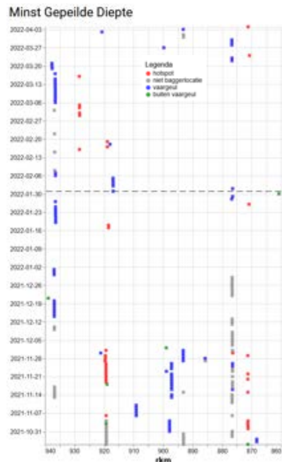
Figure 3: Visualisation of the Least Available Depth (Minst-gepeilde Diepte) along the Boven-Rijn and Waal.
